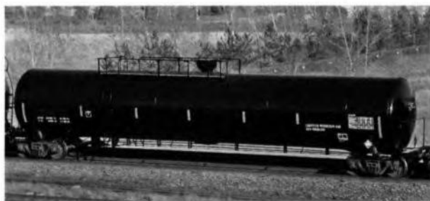
Figure 3-19 Pressurized rail tank cars have top mounted fittings for loading and unloading.
