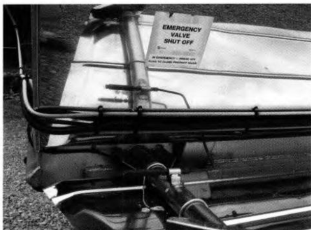
Figure 11-8 The remote shut-off valve is typically found near the front of the cab, adjacent to the driver's door, or at the rear of an MC-307/DOT-407 cargo tank.
