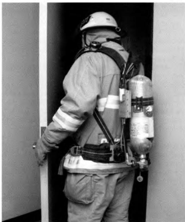
Figure 4-17 SCBA carries its own air supply, a factor that limits the amount of air and time the user has to complete the job.
