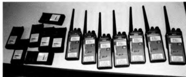
Figure 5-3 All intrinsically safe radios and batteries will be marked by the factory with a specific label denoting them as such.
