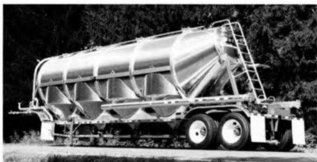
Figure 3-17 A dry bulk cargo tank carries dry goods such as powders, pellets, fertilizers, or grain.
