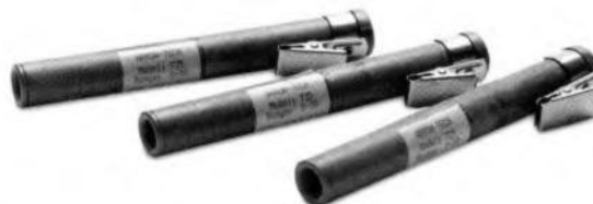
Figure 6-21 A personal dosimeter measures the amount of radioactive exposure received by an individual.
