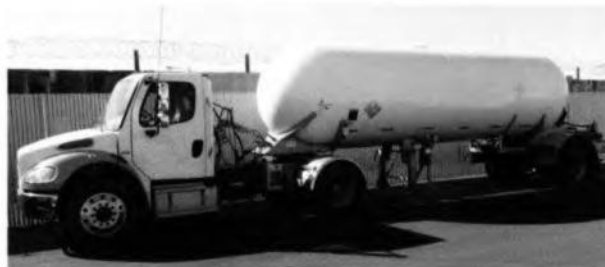
Figure 3-14 The MC-331 pressure cargo tanker carries materials such as ammonia, propane, Freon, and butane.
