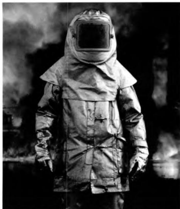
Figure 4-10 High-temperature-protective equipment protects the wearer from high temperatures during a short exposure.
