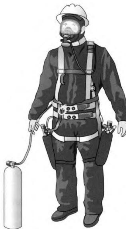
Figure 4-18 A supplied-air respirator is less bulky than an SCBA but is limited by the length and structural integrity of the air hose.
