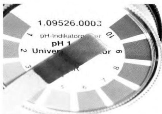
Figure 4-5 Litmus paper (pH strips) is used to determine the hazardous material's pH.
