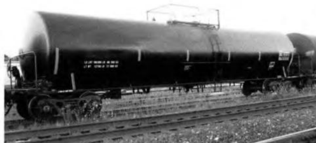
Figure 3-18 A nonpressurized rail tank car has visible valves and piping.
