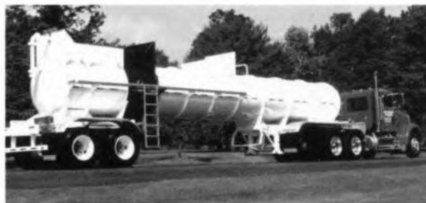
Figure 3-13 The MC-312/DOT 412 corrosives tanker is commonly used to carry corrosives such as concentrated sulfuric acid, phosphoric acid, and sodium hydroxide.
