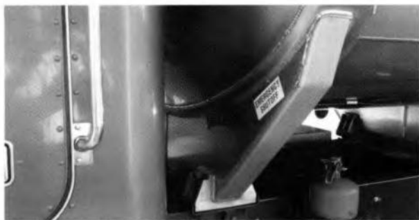
Figure 3-11 The MC-306/DOT 406 cargo tanker has a remote emergency shut-off valve as a safety feature.
