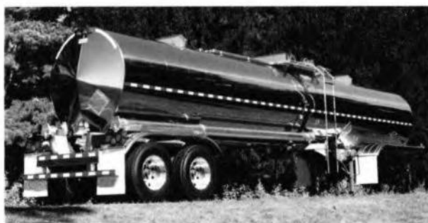
Figure 3-12 The MC-307/DOT 407 chemical hauler carries flammable liquids, mild corrosives, and poisons.
