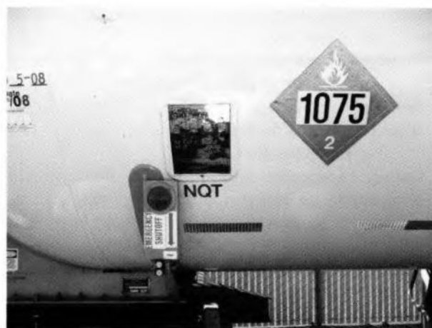
Figure 11-9 The MC-331 cargo tank has remote shut-off valves at both ends of the tank, internal shut-off valves, a rotary gauge depicting product pressure, and two top-mounted vents.
