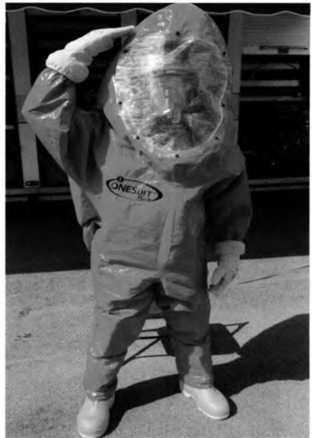
Figure 7-9 A Level A ensemble envelops the wearer in a totally encapsulating suit.
