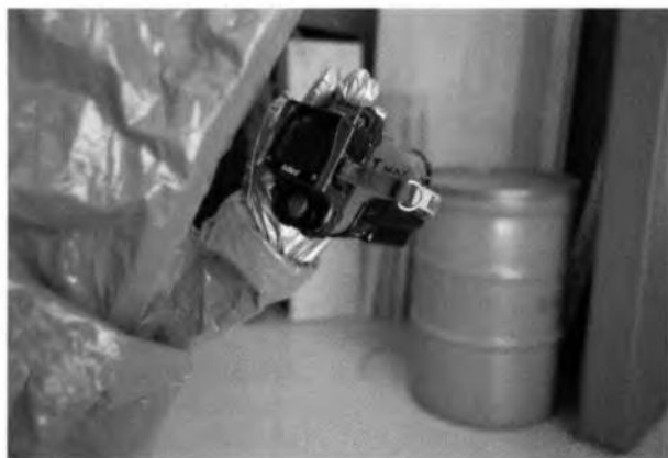
Figure 4-2 Thermal imaging cameras allow responders to estimate how much material remains in a container.
