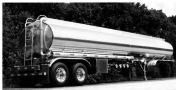
Figure 3-10 The MC-306/DOT 406 flammable liquid tanker typically hauls flammable and combustible liquids.
