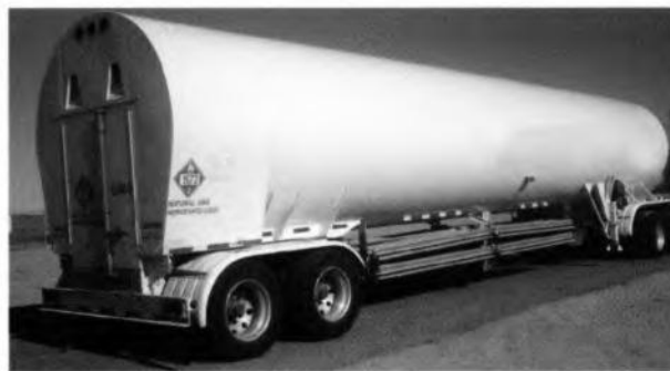
Figure 3-15 The MC-338 cryogenic tanker maintains the low temperatures required for the cryogenics it carries.
